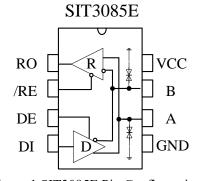
Figure 1 SIT3085E Pin Configuration
