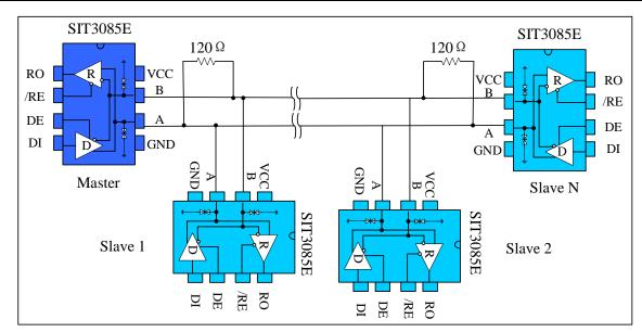
Fig 11 Bus type RS485 half-duplex communication network
