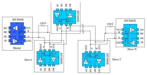
Fig12 Hand in hand RS485 half-duplex communication network
