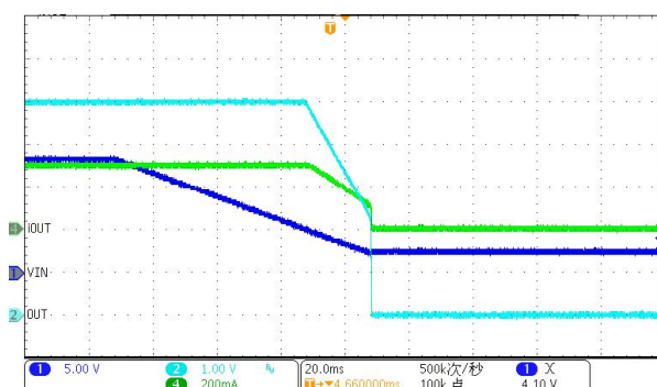
Power-OFF @ Vin=14V, Vout=5V, load=300mA
